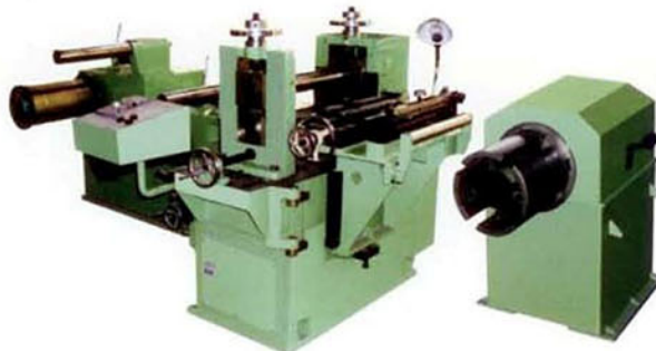
JMGJ450型滚剪纵切机 JMGJ450 longitudinal shear rolling machine
